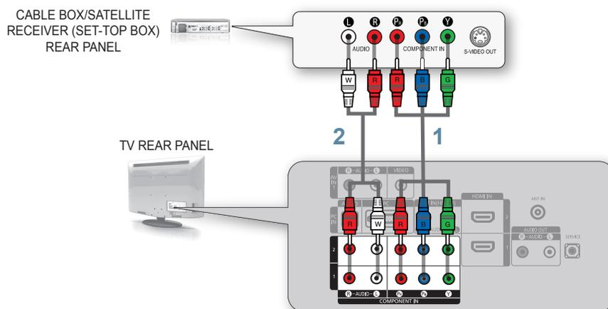
1. Connect a Component Cable(Not supplied) between the **COMPONENT IN (1 or 2) [Y, P<sub>B</sub>, P<sub>R</sub>]** jacks on the TV and the COMPONENT jacks on the Cable Box/Satellite receiver (Set-Top Box).
